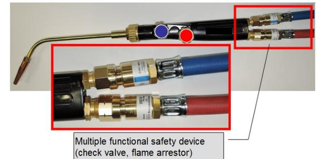
elements: check valve (non-return valve) and sintered flame arrestor.
