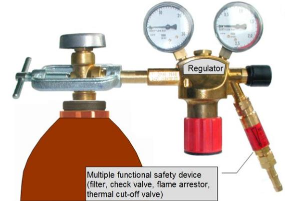
To prevent a reverse flow and a flashback, safety devices shall be mounted on the regulator and on the torch. This rule applies for both acetylene and oxygen.
